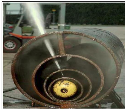
Figure 26: Cutting operation by abrasive water jet (PROSERV OFFSHORE, 2009)
